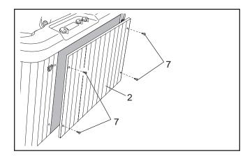
To re-attach the access panel (2), insert the top of the access panel under the edge of the spa shell. Slide the access panel up until the bottom of the access panel clears the trim along the bottom of the spa. Then, slide the access panel into place and re-attach the four #10 x 2" Sheet Metal Screws (7).
